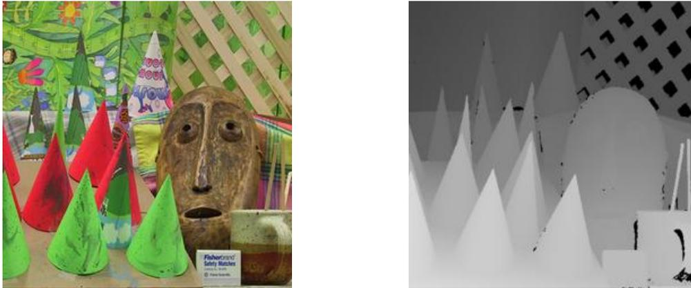
**Figure 1.** Example image (left) and the corresponding depth image (right). A typical depth image contains regions of linear depth changes bounded by sharp discontinuities.
